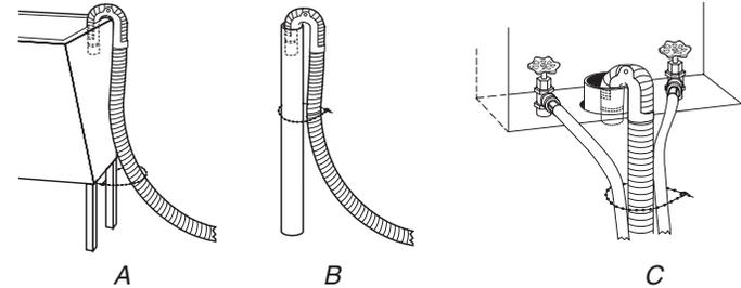
4. If the washer faucets and the drain standpipe are recessed, put the hooked end of the drain hose in the standpipe as shown. See illustration C.
