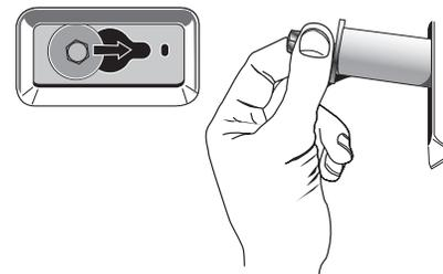
4. Once all 4 bolts are removed, discard the bolts and spacers. Then pull the power cord through the opening of the rear panel and close the hole with the attached cap.
