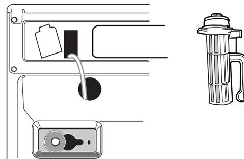
1. Keep the washer in the upright position while removing the blue bolts.
